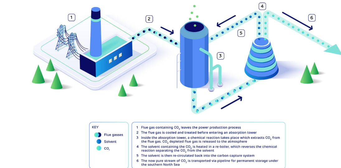
Figure 7: How carbon is captured from an emission source
